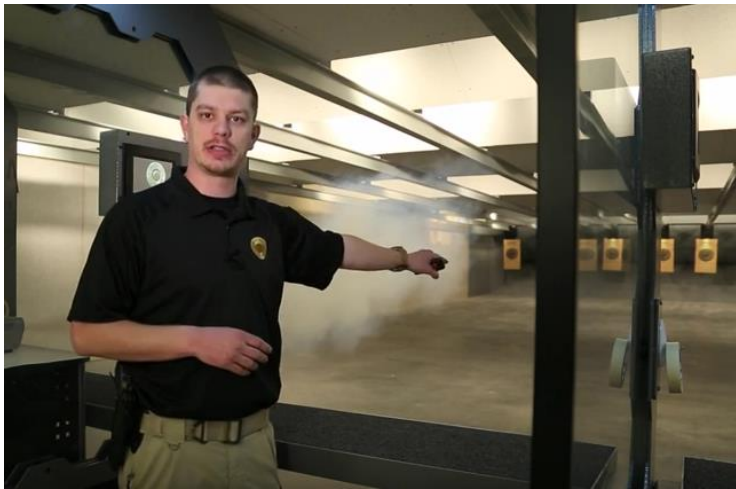
Fog machine tests the ventilation at Centennial Gun Club – “As you can see, it’s all continuing down range.”
